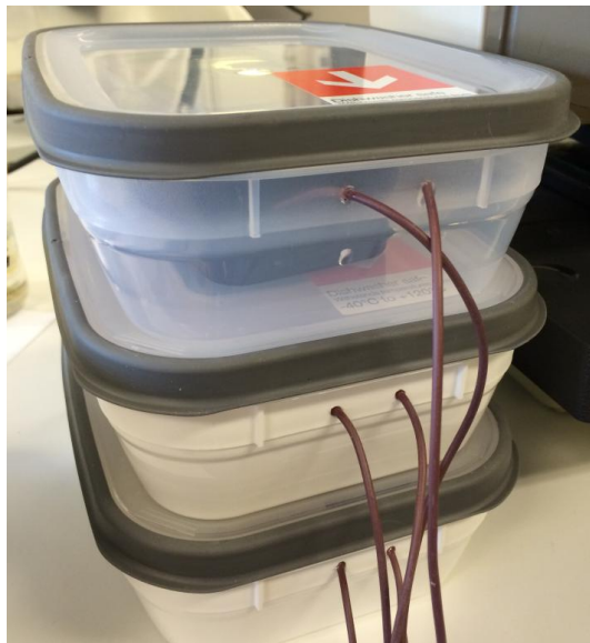
Picture 4: Three alarm clock mounted inside plastic containers showing the electrical cords exiting the side of the container. Glue around the cords, both inside and outside.
