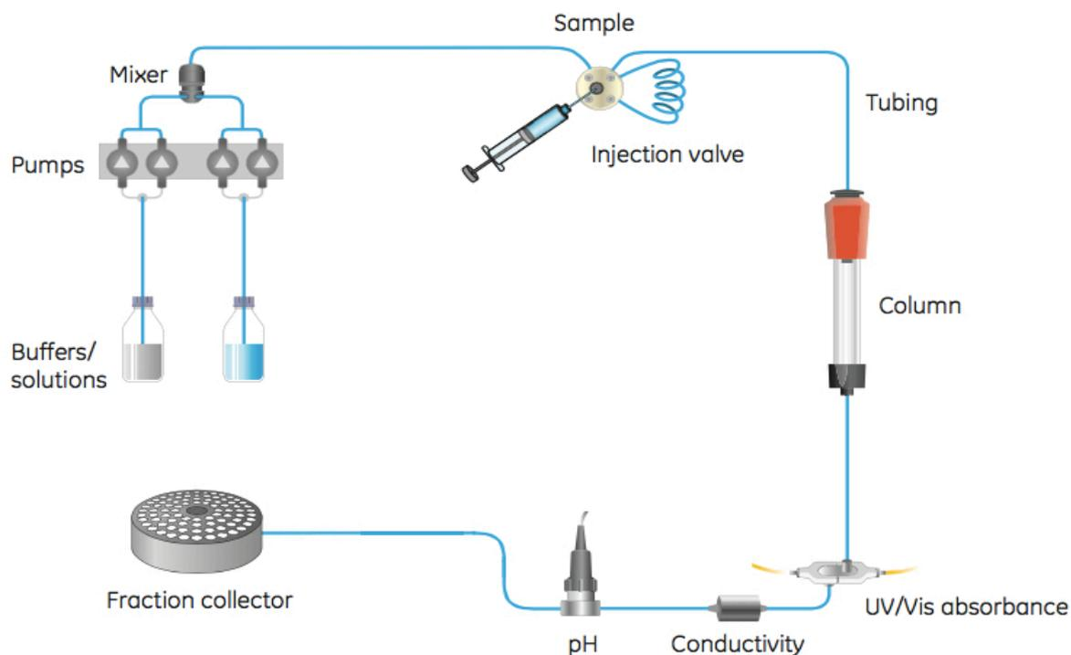
Figure 13: Typical flow path of a chromatography system (ÄKTA Laboratory-scale Chromatography Systems by GE Health care).
