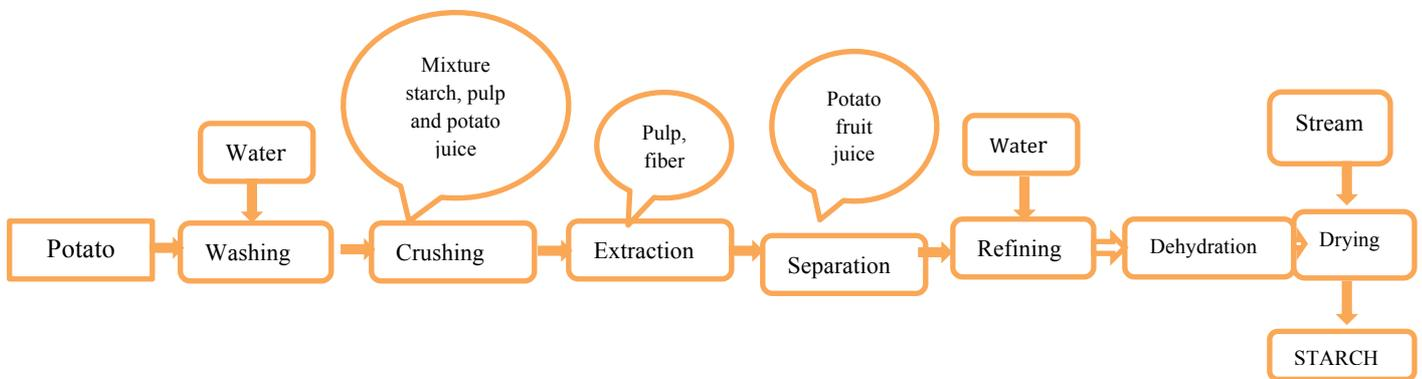
Figure 5: Potato starch manufacturing process at HOFF SA, Brumunddal, Norway. Potato fruit juice is obtained as the aqueous phase after separation by centrifugation of the denser starch material (Adapted from Løkra and Strætkvern, 2009).
