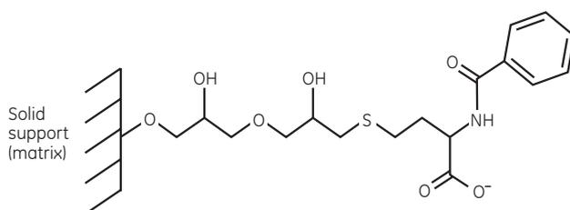
Figure 10: Capto MMC ligand structure (GE Healthcare -Data file11-0035-45 AB).
