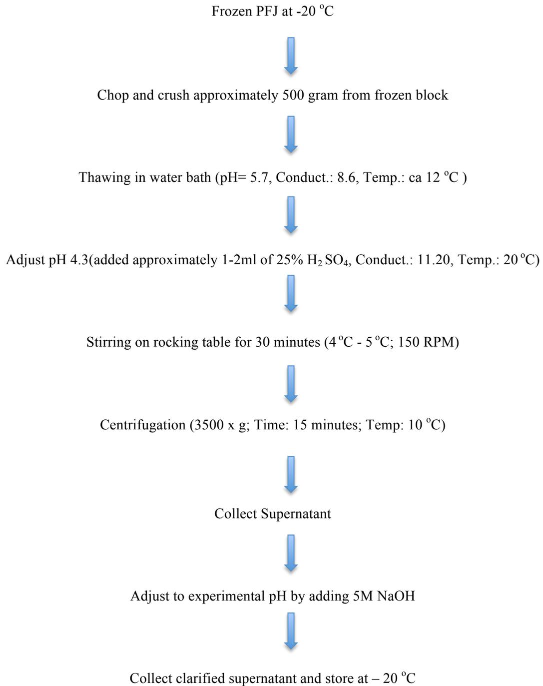
Figure 9: Preparation procedure of CAP from crude PFJ.
