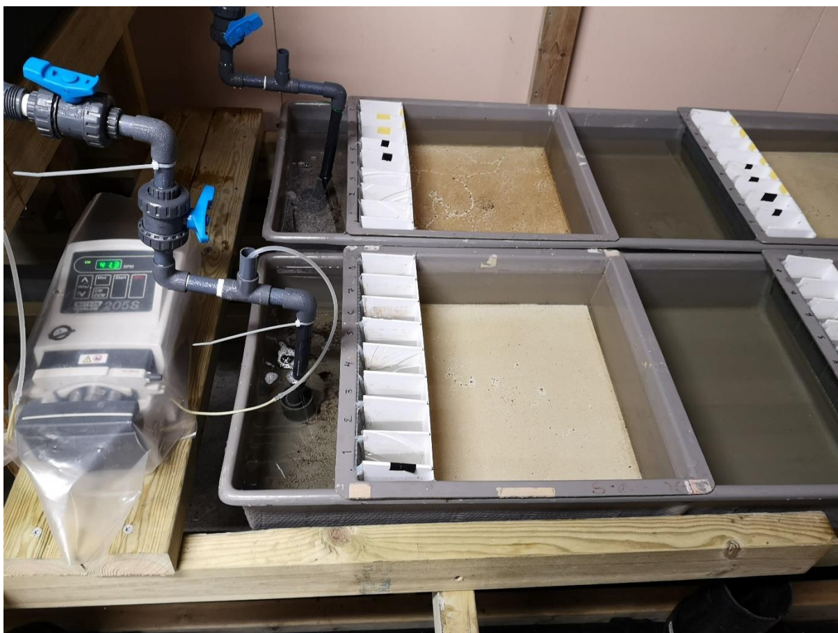
Figure 5. The stock solution is pumped with a peristaltic pump through the riser on top of the supply pipe in a silicone tube. Water and stock solution are then mixed thoroughly in the mixing cup at the bottom of the exposure channel. Further, the different media flow through the exposure chambers (white sections inside insert trays). Ball valves are visible as blue knobs on the supply pipe.
