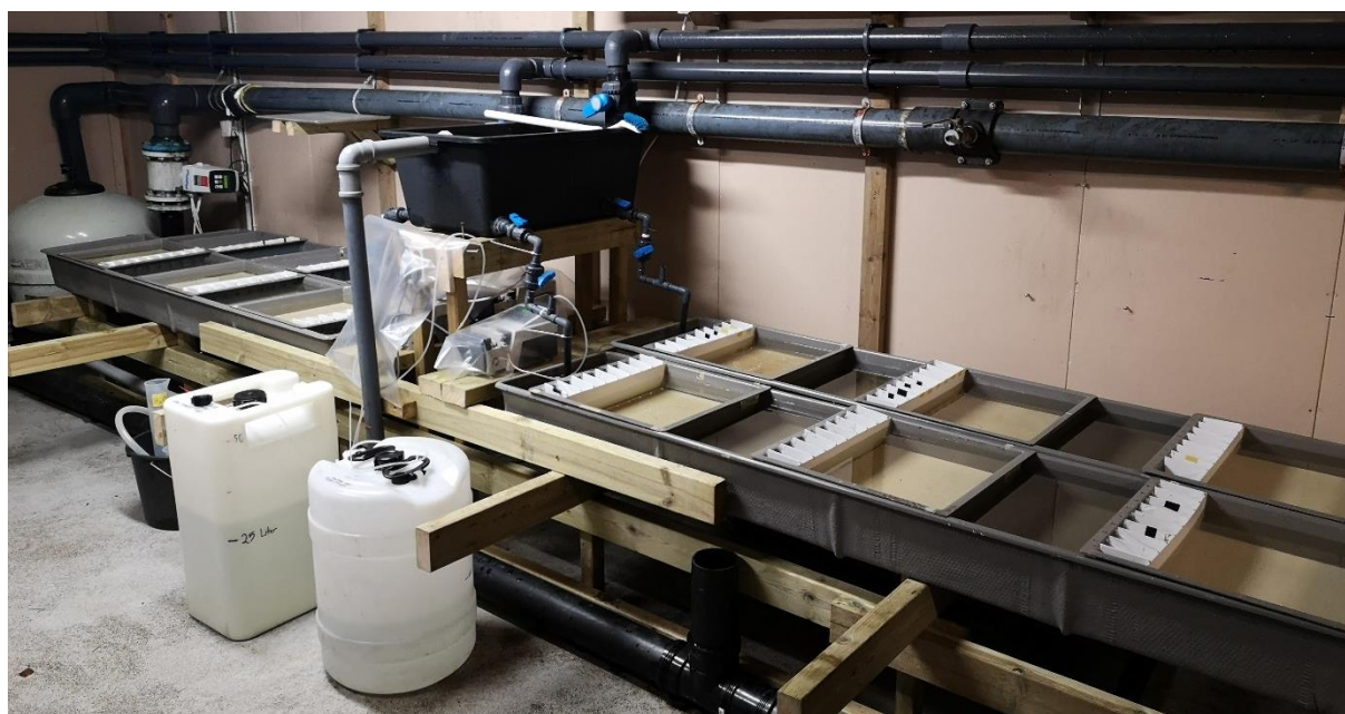
Figure 3. Overview of the experimental setup. Three Levels with one row of exposure chambers (white) were placed inside each exposure channel. White tanks contain \text{Al}(\text{NO}_3)_3 (left) and \text{HNO}_3 (right) stock solution used in the experiments. In the middle of the photo, above the channels, is the level tank with overflow (grey pipe)- and supply pipes (on the side).
