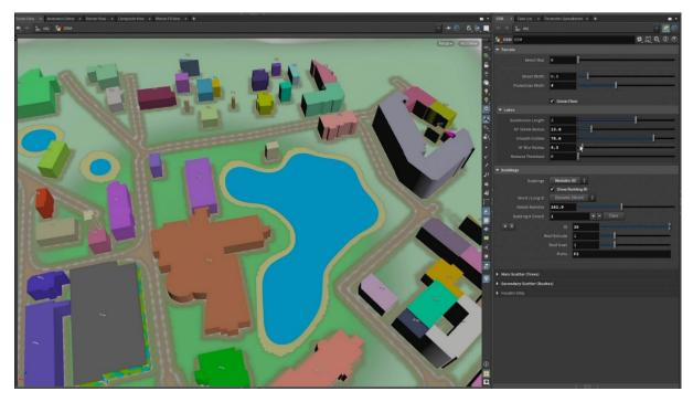
**Figure 2.** Basic three-dimensional city structure generated by the HDA from OSM data with parameter interface. Screenshot from SideFX Houdini.
