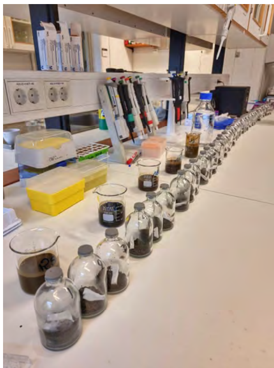
Figure 13: The lab-fertilized soil samples, incubated as agitated soil slurries, are being prepared to assess the impact of different fertilizers on soil nitrification.
