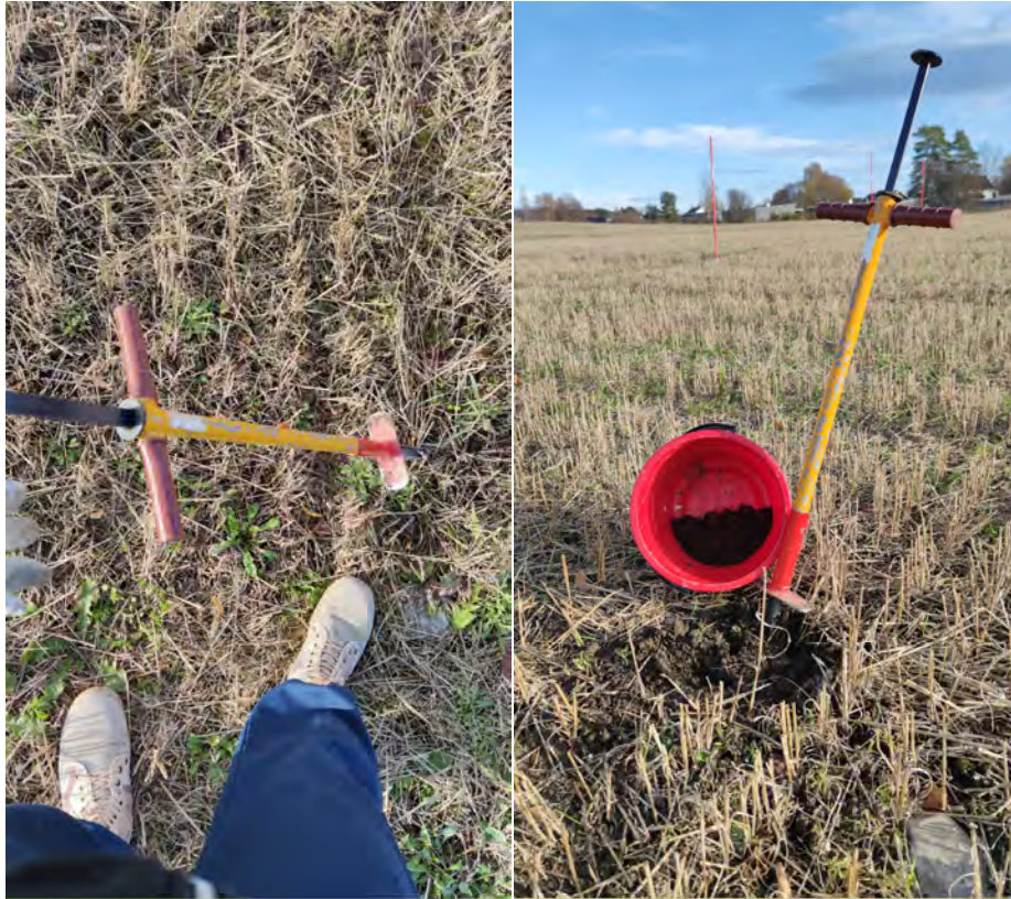
Figure 11: A corer was utilized to collect samples from the experimental plots treated with different fertilizers. Ten representative samples were extracted diametrically from each plot replicate.
