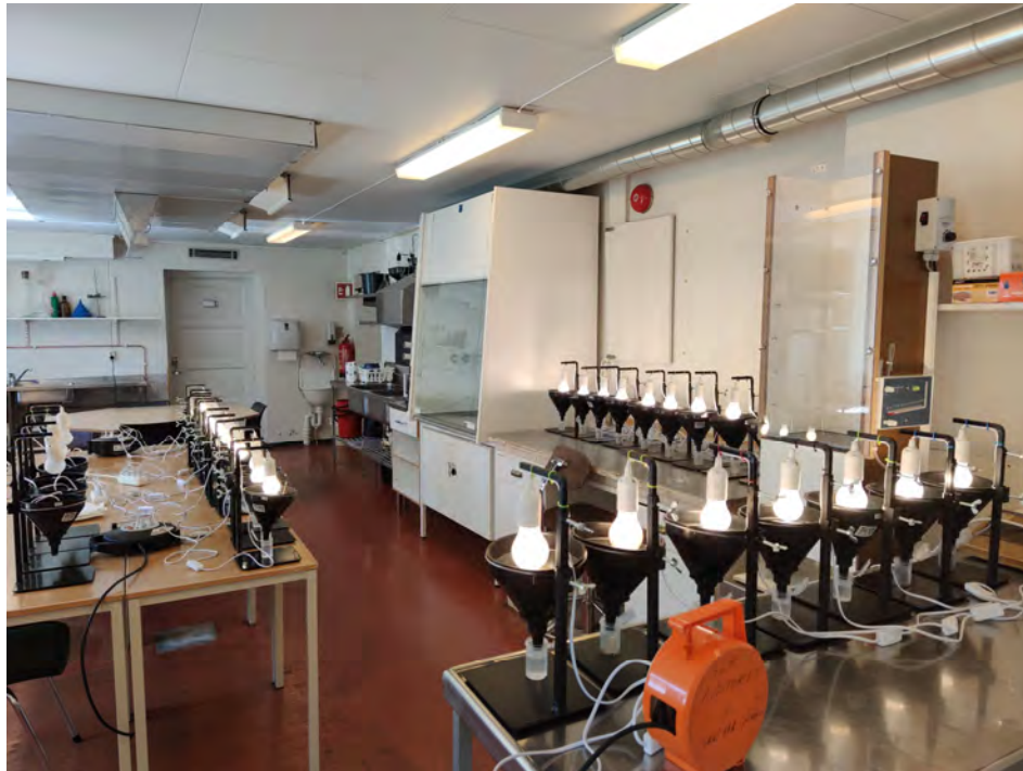
Figure 9: Experimental setup using Tullgren funnels to extract springtails from soil samples collected at each sampling occasion.
