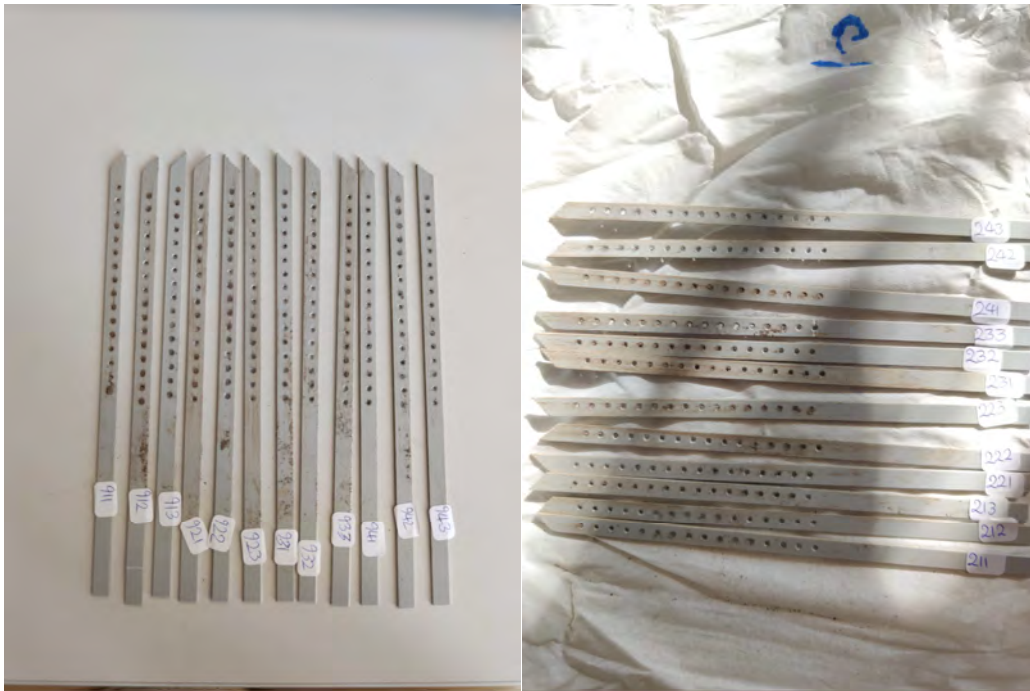
Figure 16: Examples of Bait-lamina strips with consumed bait material; each empty hole represents 6.25% soil fauna feeding activity.
