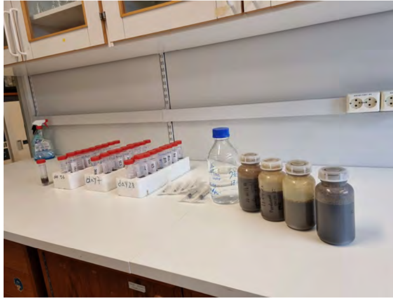
Figure 14: The lab-fertilized soil samples, incubated as loose soil, are being prepared to assess the impact of different fertilizers on soil nitrification.
