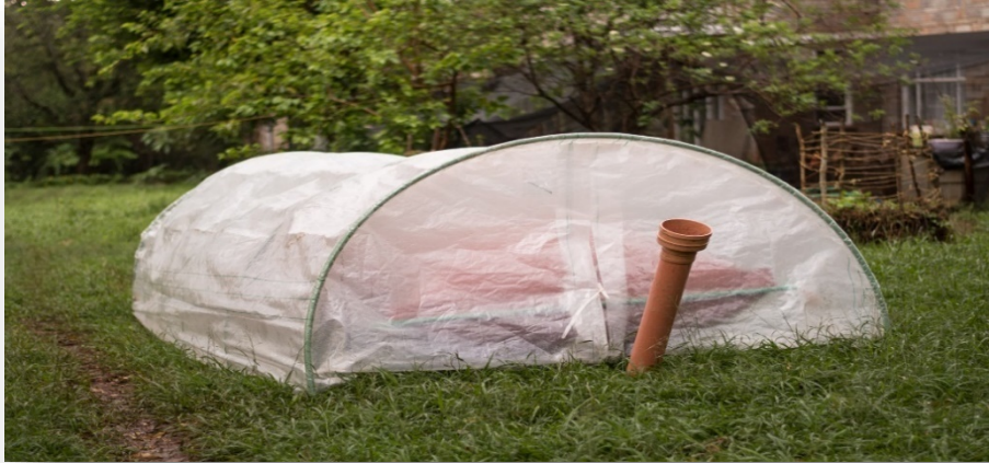
Figure 6 The prototype of a tubular micro biogas digester
