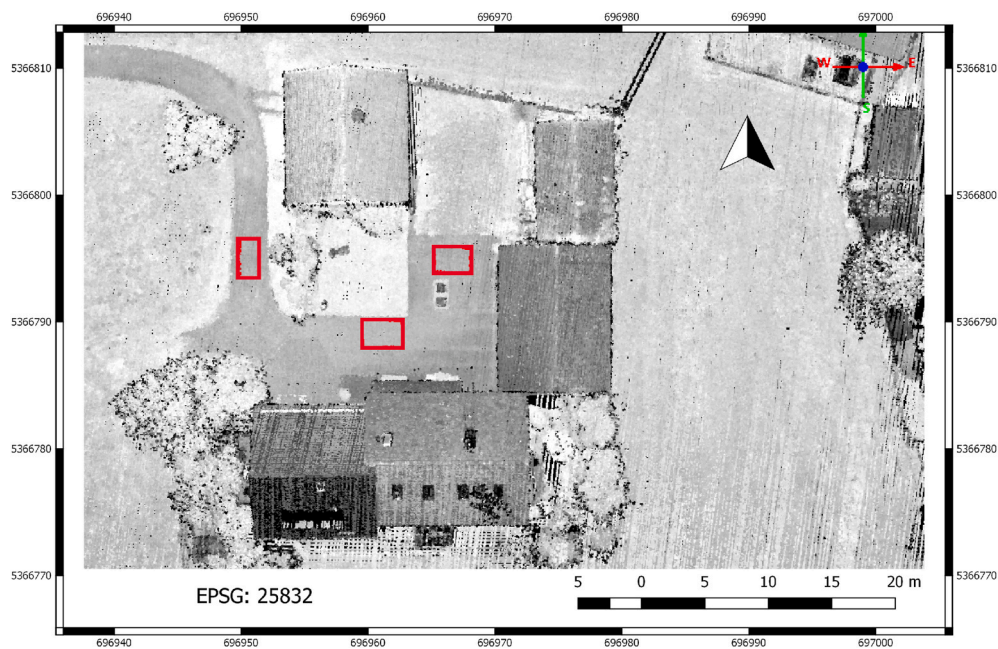
Fig. A1. Three small concrete areas (red polygons) providing mean values I_n for calibration of lidar intensity.
