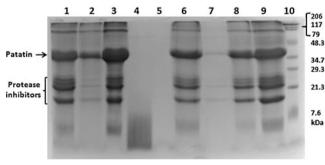
**Fig. 4** Coomassie-stained SDS-PAGE (15%) analysis of fractions from EBA and UF processing steps. *Lane 1–4*, EBA: *1*, crude PFW; 2, flow through; 3, eluate; 4, regeneration. *Lane 5*, empty. *Lane 6–9*, UF: 6, crude PFW; 7, permeate; 8, retentate 10× dil.; 9, retentate 5× dil.; 10, molecular weight markers (BioRad Broad Range)
