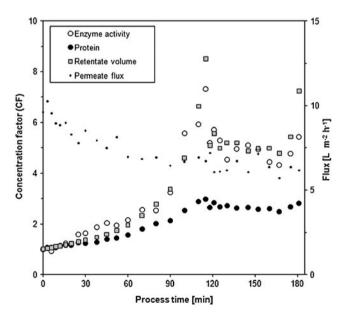
Fig. 3 Batch concentration and diafiltration of 2.4 1 PFW using ultrafiltration with 10-kDa MWCO. *Data points* indicate the effect of volume reduction on the concentration of protein (*closed circles*), esterase activity (*open circles*), retentate volume (*open squares*), and change in permeate flux (*small dots*). Onset of diafiltration with distilled water was at 118 min
