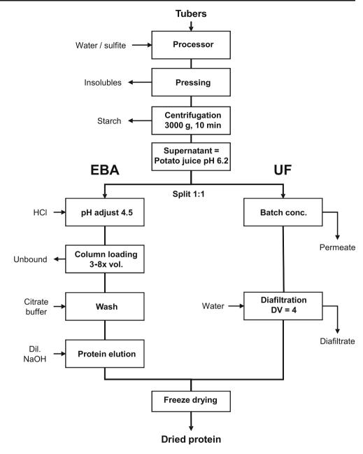
concentration was stopped when the reservoir level was ca. 70 ml; the system holdup volume was approximately 250 ml, thus a total retentate volume of approximately 320 ml.
