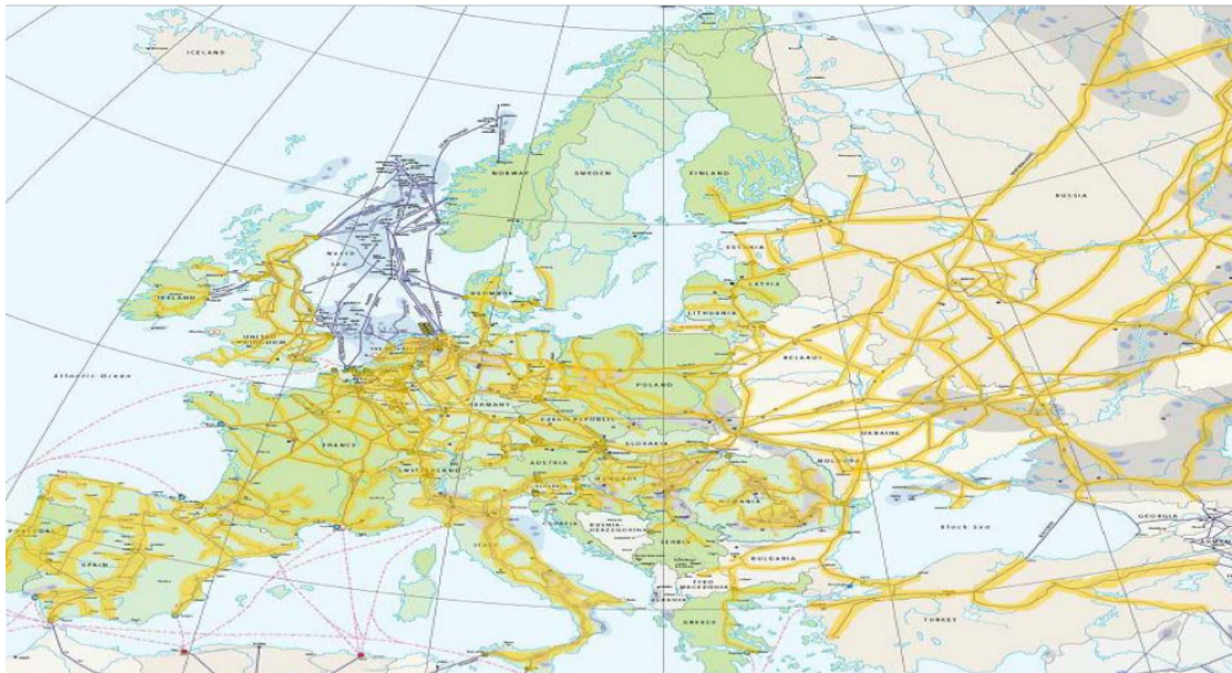
Figure 2 Potential corridors for biogas production (yellow) in Europe and supply in natural gas grid (Thrän et al., 2007)
