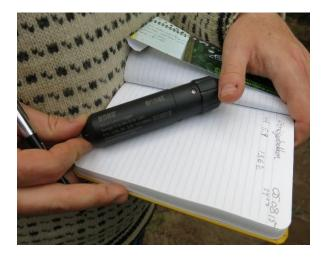
Figure 12: HOBO U20L, barometric pressure and water temperature data logger. This device was set to record water temperature and barometric pressure once pr. hour. This yielded an expected battery life of > 2 years. The device was placed under water and mounted to the water level gauge.
