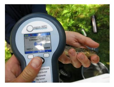
Figure 17: Handheld PIT-tag reader. With the handheld reader, the number of the PIT-tag placed inside the abdomen of brown trout could be read. The long number on the display is the number of the PIT-tag.
