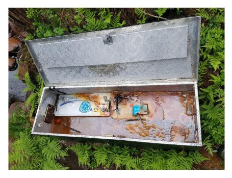
*Figure 38: A flood has filled the antenna station with water in tributary D in summer 2016.*
