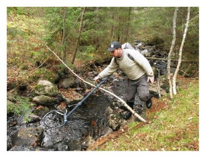
Figure 15: Backpackreader operator in action. The portable antenna system is used to account for marked brown trout still residing in the tributary. The extended plastic tube, with a loop in the end is the antenna, while the registration system and batteries are carried in a small backpack.
