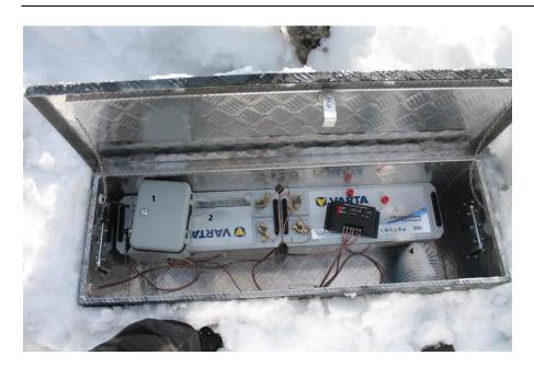
Figure 14: The inside of the aluminium box containing the PIT-tag antenna registration station with the following components 1: PIT-tag registration box, 2: batteries, 3: Solar panel regulator box, 4: Dehumidifier to reduce humidity inside the box.
