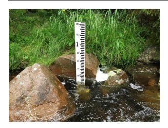
Figure 11: A water level gauge was mounted in a small pool to have a reference point on water levels. The gauge was bolted into rock, to make it withstand floods and debris. The same equipment was mounted in each of the four tributaries.
