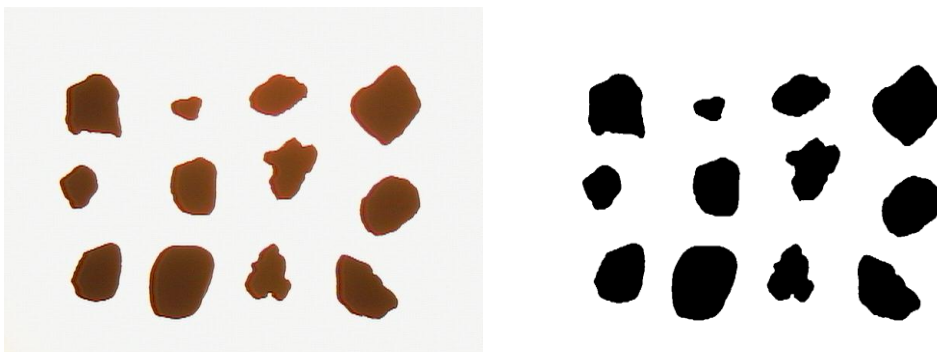
Figure 3. Images of rock ptarmigan grit for analysis in the software Morphocop. Left, an image from the digital camera; right, an image after processing and ready for further analysis.
