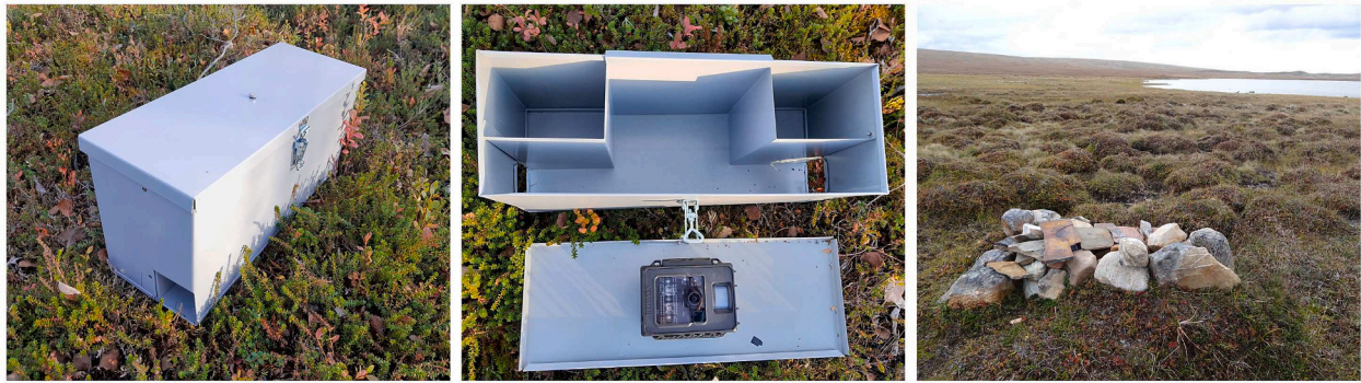
Fig. 3. The camera trap developed by Soinin et al. (2015) consists of a Reconyx camera that is mounted on the ceiling of a metal box that can be entered by small mammals. The camera traps are protected with stones when placed in the field.
