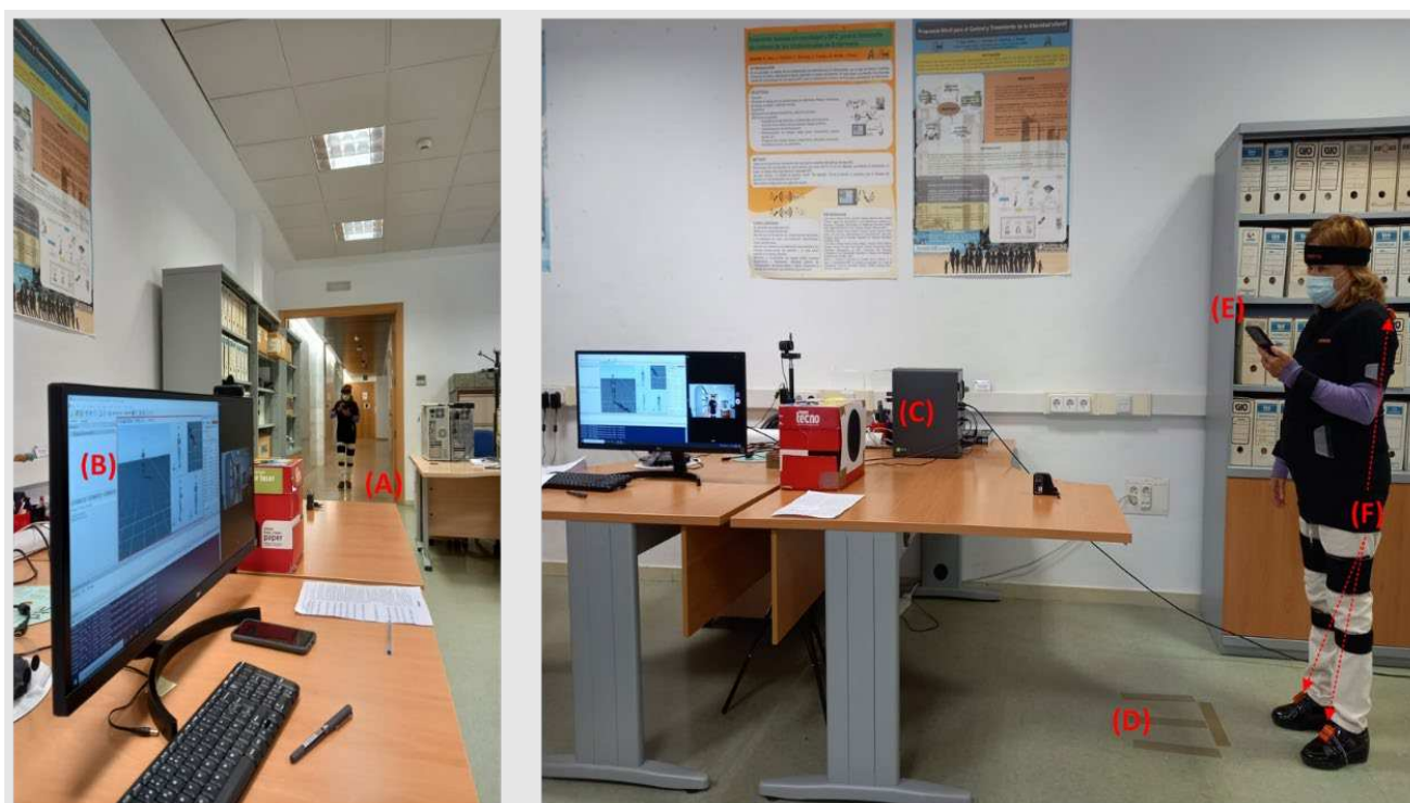
Figure 2. Instrumentation and experiment environment. (A) 24-m-long corridor the participants must walk. (B) Monitor where the movement of the person is visualized in real time. (C) Computer with motion capture software. (D) Start position marks. (E) Personal mobile device. (F) Some of the MTw IMUs.
